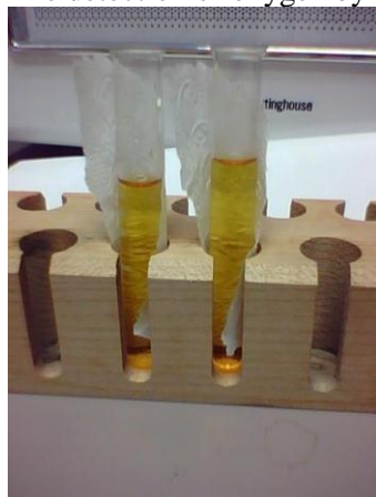
Figure 4 Photograph showing a luminescent probe species in solution with normal lighting
